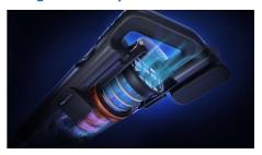
5-stage advanced filtration system filters up to 99.9% of fine dust, bacteria and allergens [10]. The filtration consists of our newest, in-line PowerCyclone 12 with Aerodynamic Vortex Blades, 3-stage foam filter package and final stage fine particle electret filter
